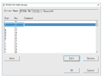
The Control A Editor is opened. Enter the ESC/POS command in hexadecimal format into the [Command] text box. After entry, click [OK].
