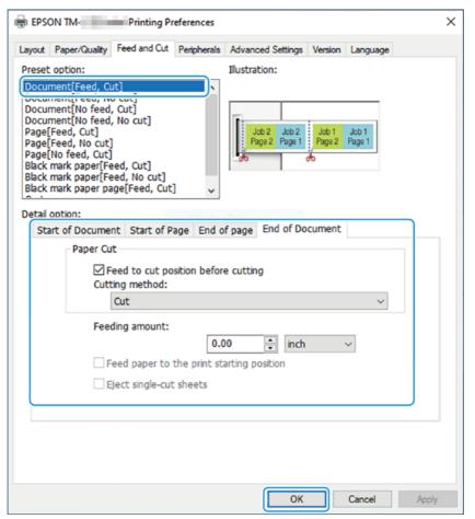
2 Select the control timing from the [Detail option] tab to set up the operation. The settings are described in the following table.
