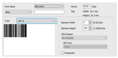
To set a variable-length barcode, enter data containing the number of columns to be printed in [Test Printing].
