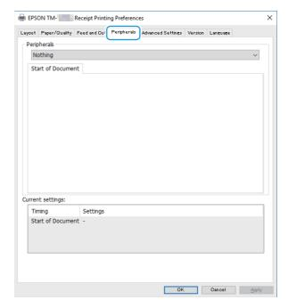
From the [Peripherals] pull-down list, select the combination of peripheral devices to be connected to the TM printer.
