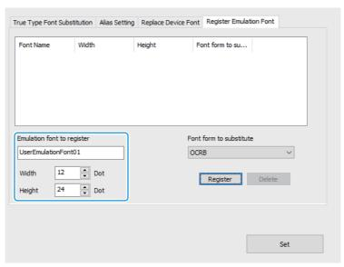
Select a TrueType font to be replaced from the [Font form to substitute] pull-down list, and click [Register].
